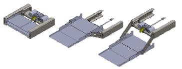
The operational sequence of the lift includes mainly two phases: the platform extraction and its vertical movement until reaching the desired boarding level.
