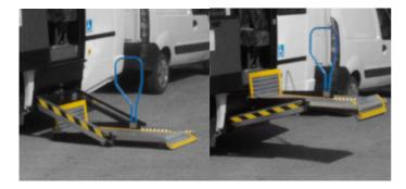
An example of cars application with the vertical motion of the loading platform electrically driven and a semi automatic platform extraction.
