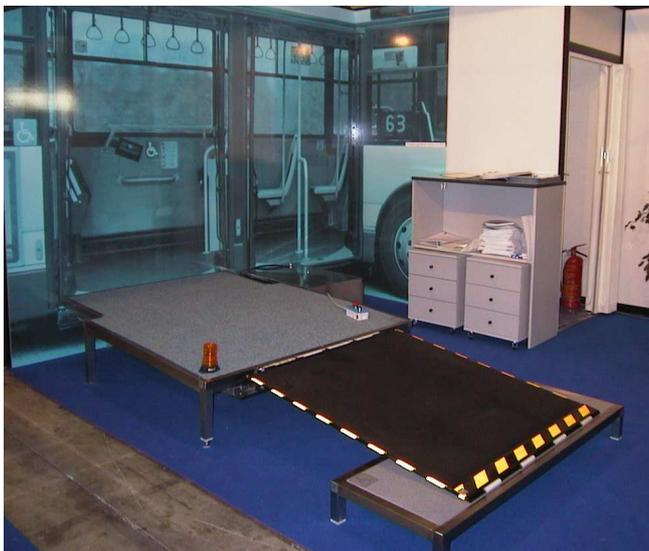
A prototype of the new generation ramp with innovative features and suited to the rugged northern environmental conditions, will be installed on a NSB Class 72 vehicle.
